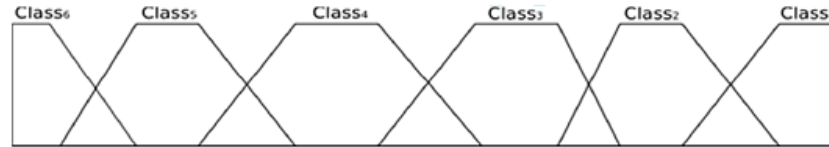
Fig. 9. The classes based on fuzzy trapezoidal membership functions.
